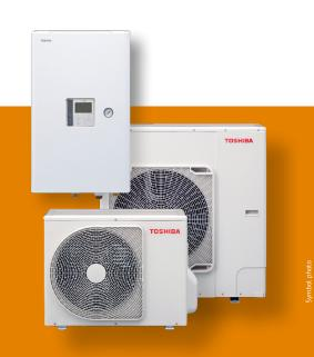
R32 Air to water heat pumps in split design for leaving water temperatures up to +65°C, in the capacity range from 4 to 14 kW, for the preparation of hot or cold water. Combination of outdoor unit and hydrobox to supply all applications such as hot water tanks, fan coils, radiators or underfloor heating.
